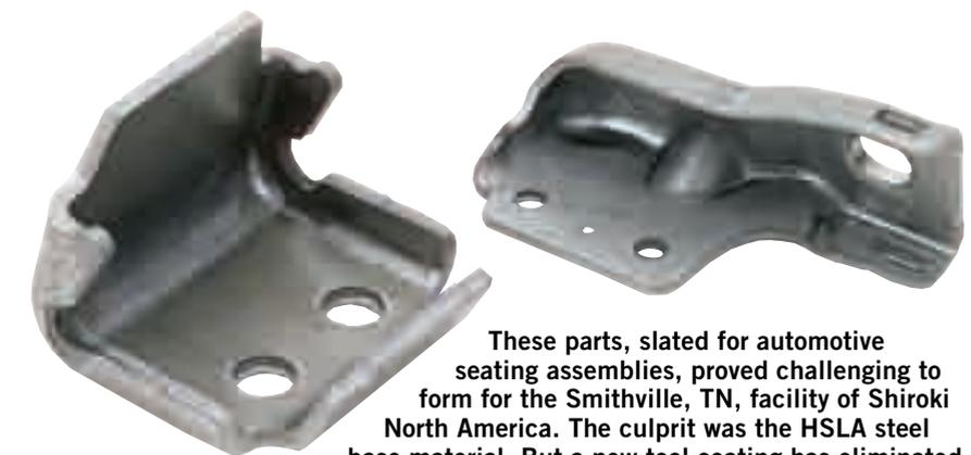
These parts, slated for automotive seating assemblies, proved challenging to form for the Smithville, TN, facility of Shiroki North America. The culprit was the HSLA steel base material. But a new tool coating has eliminated galling and cut part-rework time and expense.
