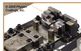
Glacier recently began assigning part numbers to elements of its quick change tooling. The shinier sections to the right are polished and coated with Phygen's FortiPhy CrN coating.
