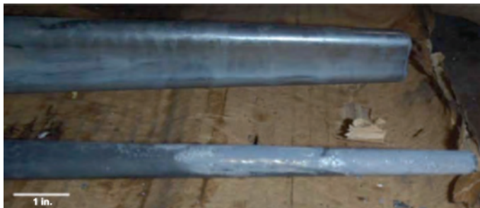
Fig. 5 — Steel slide inserts used in the production of a die cast driveshaft housing after 1256 shots [4] . The upper core with a 5-µm thick AlCrN coating shows no soldering, while the lower uncoated insert shows soldering.
