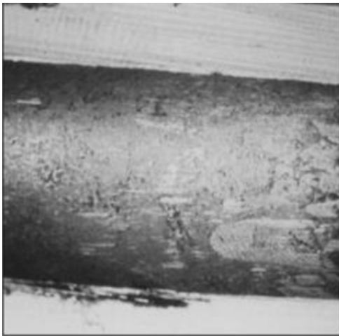
Figure 1 – Solder on the surface of a core pin.
