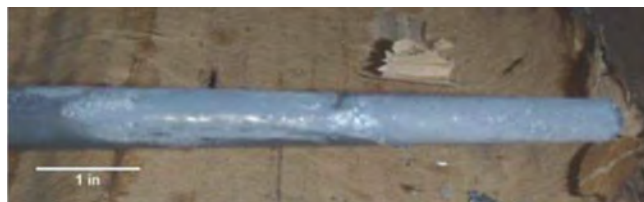
Figure 5 - Solder build-up on un-coated core. 11
