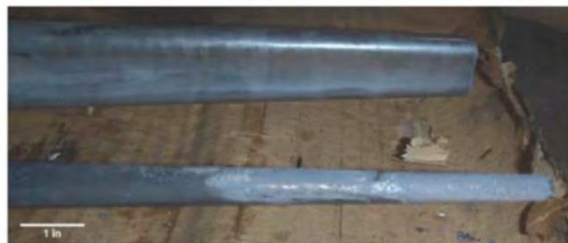
Figure 6 - Comparative photo of two slide inserts after 1,256 shots. The upper insert was treated with CertiPhy Plus and shows no soldering, while the lower (soldered) insert was un-coated. 11
