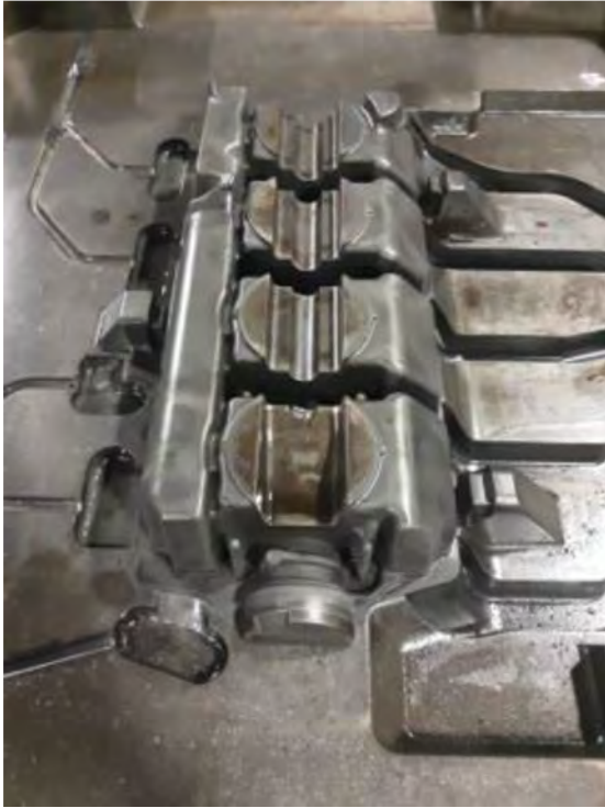
Figure 2 - Cavity insert for rod well for Mercury 4-cylinder engine blocks (photograph by Phygen).
