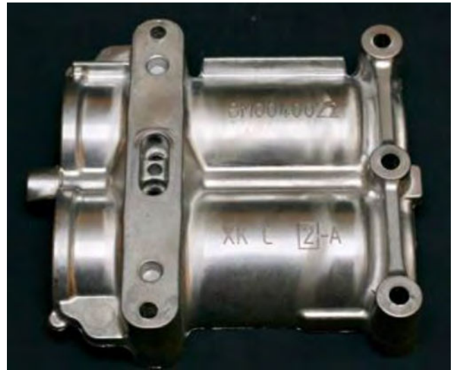
Figure 7 - Photograph of the balance shaft housing after more than 70,000 castings have been produced in the die (photograph by Phygen).
